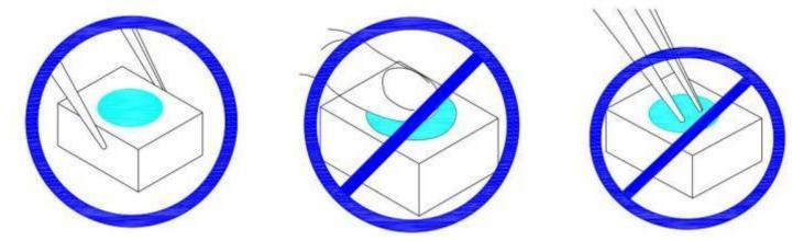
2.2 Do not stack to get her assembled PCBs containing LEDs. Impact may scratch the silicone lens or damage the internal circuitry.
