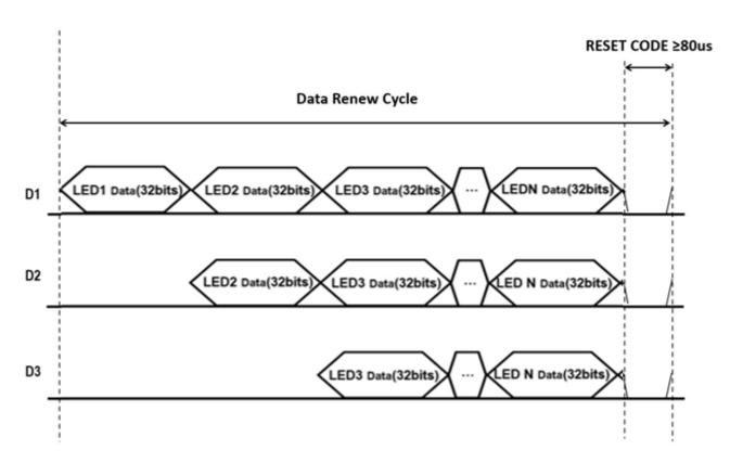
Note: D1 is the data sent by the MCU, and D2, D3, and D4 are the data that the cascade circuit automatically reshapes and forwards.
