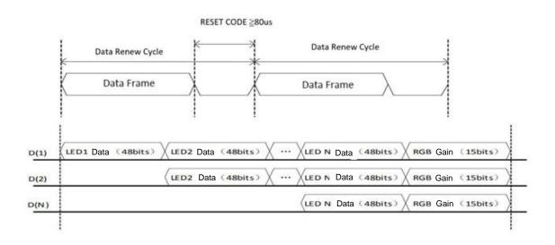
Note: Data frame D(1) is the data sent by MCU .D(2) and D(N) are the data automatically shaped And forwarded by the cascade circuit.
