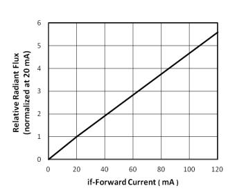
Fig.1 - Relative Radiant Flux vs. Forward Current
