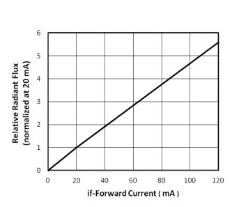
Fig.1 - Relative Radiant Flux vs. Forward Current
